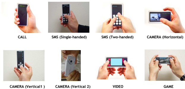
Figure 7: Defining 8 grip patterns for 5 mobile device applications
