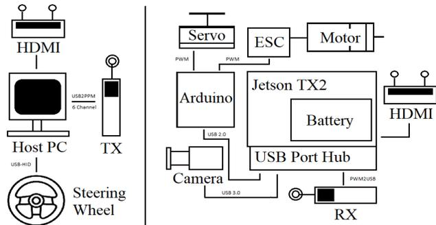
Fig. 2. Hardware System Architecture: An HDMI digital wireless transmitter minimizes latency with a gaming monitor at sub 11ms. An Nvidia Jetson TX2 board was used as the embedded processor. A CMOS camera with 185 degrees field of view (FOV) provided images at 80 frames-per-second (FPS).
