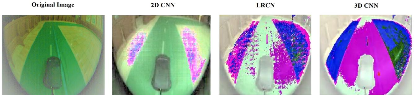
Fig. 5. Salient feature activations (purple) for different neural network architectures. Based on the amount of salient feature activations on the given image, 3D-CNN best distinguishes lanes from cars and from the road external environment.
