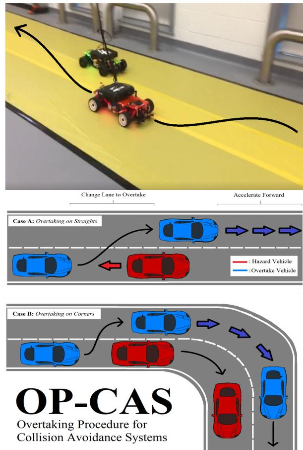
Fig. 1. **OP-CAS: Overtaking Procedure Collision Avoidance System** This collision avoidance system uses an overtaking procedure for various highway collision scenarios, as shown in Case A: "Overtaking on Straights" and Case B: "Overtaking on Corners"
