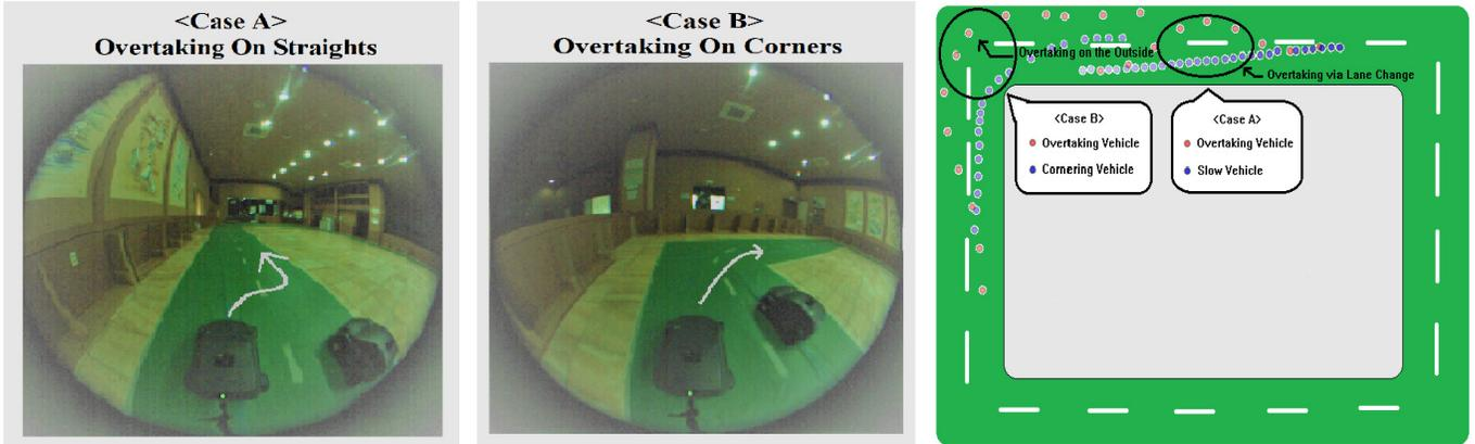
Fig. 4. Overtaking procedures used for *OP-CAS*: *OP-CAS* accounts for two cases of different overtaking maneuvers. The map on the right overlays the trajectory of the overtaking vehicle (red) and the vehicle that is being overtaken (blue).
