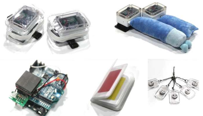
Figure 1. Components of the prototypes: a) flex sensors, b) light sensors, c) RFID reader without the enclosure, d) card type RFID tags, e) coin type RFID tags. (Counter-clockwise from the top right)
