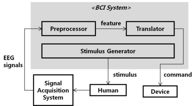
Figure 2. A typical architecture of the P300-based BCIs.
