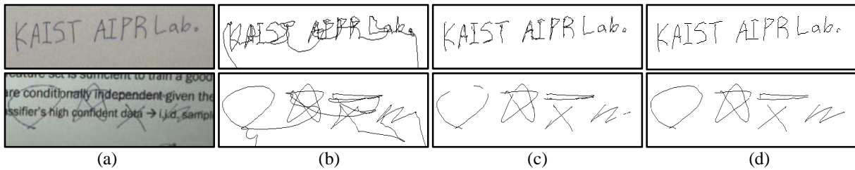
Figure 6. Examples of classification result. (a) Images after writing. (b) Complete pen trajectories. (c) Local classification results. (d) Global correction results.
