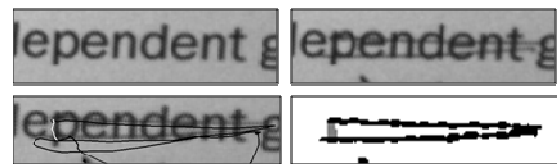
Figure 7. Example of hidden ink restoration error. Each image shows the reference image, the image after writing, the complete pen trajectory and the written ink image, respectively.
